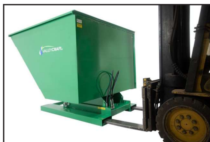
Step 1: Insert forks into fork pockets & secure unit using included safety chain.
