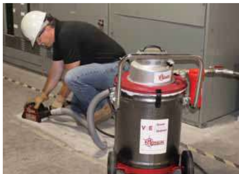
Electric model with Roto Peen tool removing coating on concrete.
