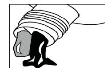
Attach mixing nozzle to the cartridge and dispense a small amount of material into the same disposable container until a consistent color, with no streaks is obtained.
