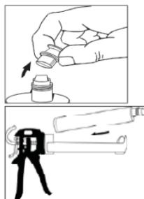
Dispense a small amount of adhesive into a disposable container until both materials are flowing evenly from the cartridge.
