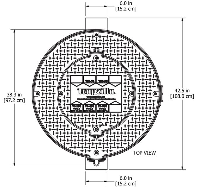
10 in [25.4 cm] CLEARANCE FROM TOP OF TANK REQUIRED FOR LID REMOVAL
