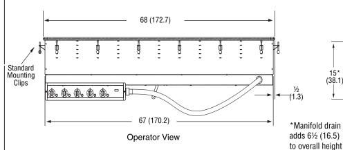
Controls must be mounted on operator (raceway) side for proper orientation with wells.
