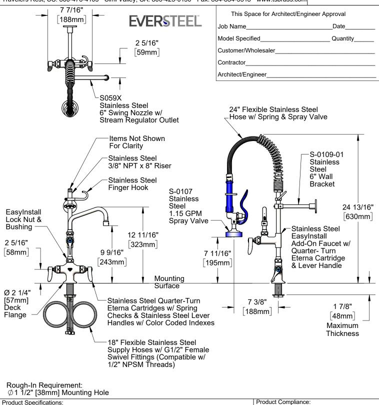
Pre-Rinse Unit: EasyInstall Stainless Steel Single Hole Deck Mount Mixing Faucet, SS Quarter-Turn Eterna Cartridges w/ Spring Checks, SS Lever Handles, SS Add-On Faucet, SS 6" Swing Nozzle, 24" Flexible Stainless Steel Hose, SS 1.15 GPM Spray Valve, SS 6" Wall Bracket & Flexible Stainless Steel Supply Hoses
