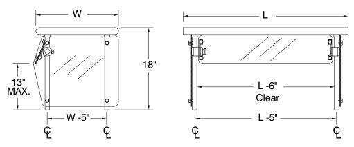
10-1/2" Standard Glass Opening (Maximum 13") From Table To Bottom Of Glass. NSF Requires Side Glass to be 18" Wide Minimum.
