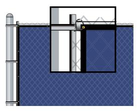
Most installations use the chain link mesh as the attachment points and not the posts, requiring only L7 Fasteners for a clean, strong fit.
