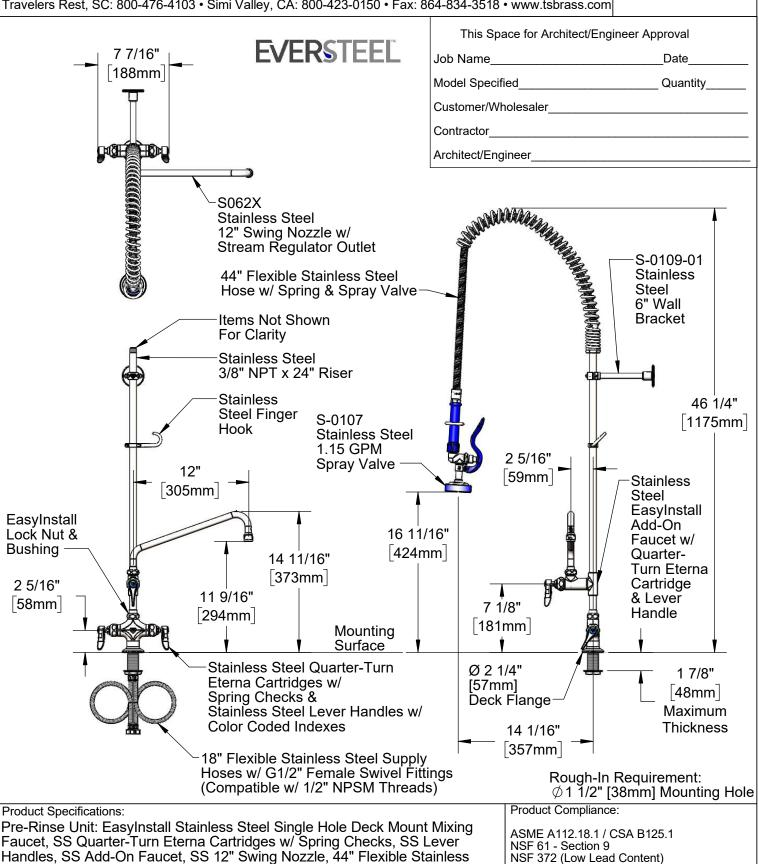
Steel Hose, SS 1.15 GPM Spray Valve, SS 6" Wall Bracket & Flexible
