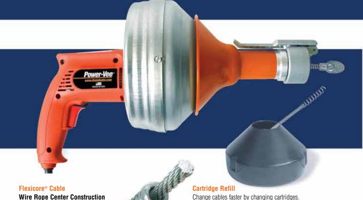
Heavy-gauge wire coiled tightly around 49-strand aircrafttype wire rope and heat treated. Has unequalled strength and the right amount of flexibility. So tough it carries a one-year warranty against defect or breakage.
