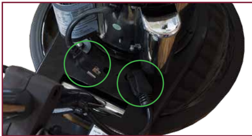
Convenient Unplug to disconnect motor for service
