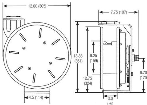
Our LE9000 series of reels are built with durable all-steel weatherproof (NEMA 4 enclosure) construction so that they will survive in the toughest work environments. We've built the cable guide arm with thicker steel than our competitors to take extra abuse. All this while still keeping the form factor small so that your reel isn't always in the way.
