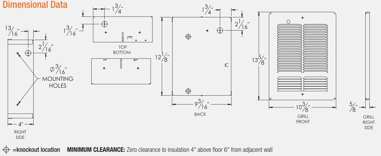
**MINIMUM CLEARANCE:** Zero clearance to insulation 4" above floor 6" from adjacent wall
