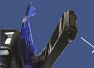
Disconnect one side at a time by gently pulling down on the tabs on either side of the ink roller.
