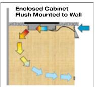
Cabinets should be sufficiently open to allow fresh air to cool the units. Two areas equal to 20 sq. inches (129 sq. cm) each should be provided for each unit. These should be located as close as possible to the intake
