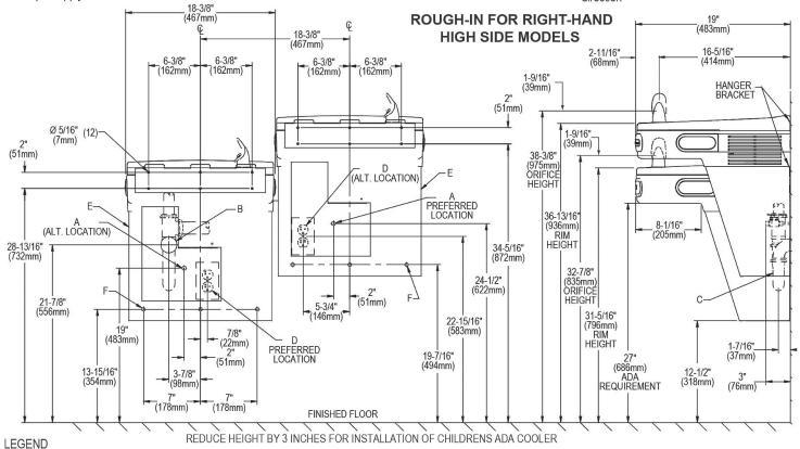
A = Recommended water supply location. Shut off valve (not furnished) to accept 3/8" O.D. unplated copper tube connect. Up to 3" (76mm) maximum out from wall. B = Recommended waste outlet location. To accomodate 1-1/2" nominal drain. Drain stub 2" (51mm) out form wall.
