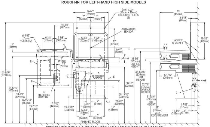
REDUCE HEIGHT BY 3 INCHES FOR INSTALLATION OF CHILDREN'S ADA COOLER LEGEND: A = Recommended Water Supply location. Shut-off Valve (not furnished) to accept 3/8" O.D. unplated copper tube. Up to 3" (76mm) maximum out from wall. B = Recommended Waste Outlet location. To accommodate 1-1/2" nominal drain. Drain stub 2" (51mm) out from wall.
