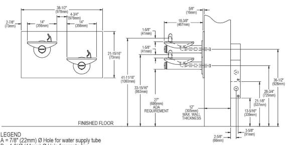
A = 7/8" (22mm) Ø Hole for water supply tube B = 1-3/4" (44mm) Ø Hole for waste line
