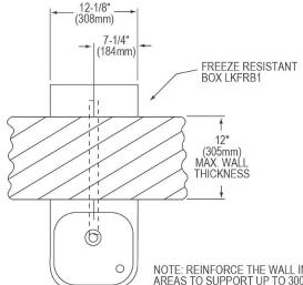
WARNING: The free-resistant box must be installed on an interior heated wall where the temperature does not drop below 50° F (10° C). The front of the box must have unobstructed air flow. Failure to maintain the interior wall temperature and the inside of the freeze resistant box above 50° F (10° C) can result in damage to the box which could result in unrestricted water flow
