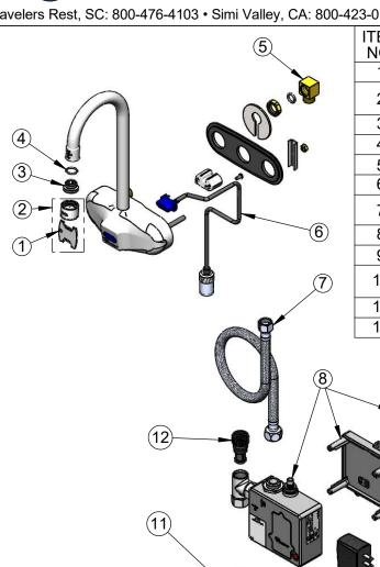
ITEM SALES NO. DESCRIPTION NO. 015425-45 Vandal Resistant Key VR Aerator, 1.2 GPM, 55/64-27 2 B-0199-06-F12 Female 3 044A 3/8" to Aerator Adapter 4 006575-45 -015 O-Ring 5 015345-45 Low Profile Elbow, 3/8 NPSM 6 017195-45 Angled Sensor with Cable 7 016325-45 Flex Connector, 3/8 NPSM x 1/2 NPSM 8 016647-45 ChekPoint Control Module (Grey) A/C Transformer 9 5EF-0002 Supply Hose, 9/16-24 Female x 1/2" 10 5EF-0005 NPSM 11 5EF-0006 Mechanical Mixing Valve 12 **EC-FILTER** Replacement Filter
