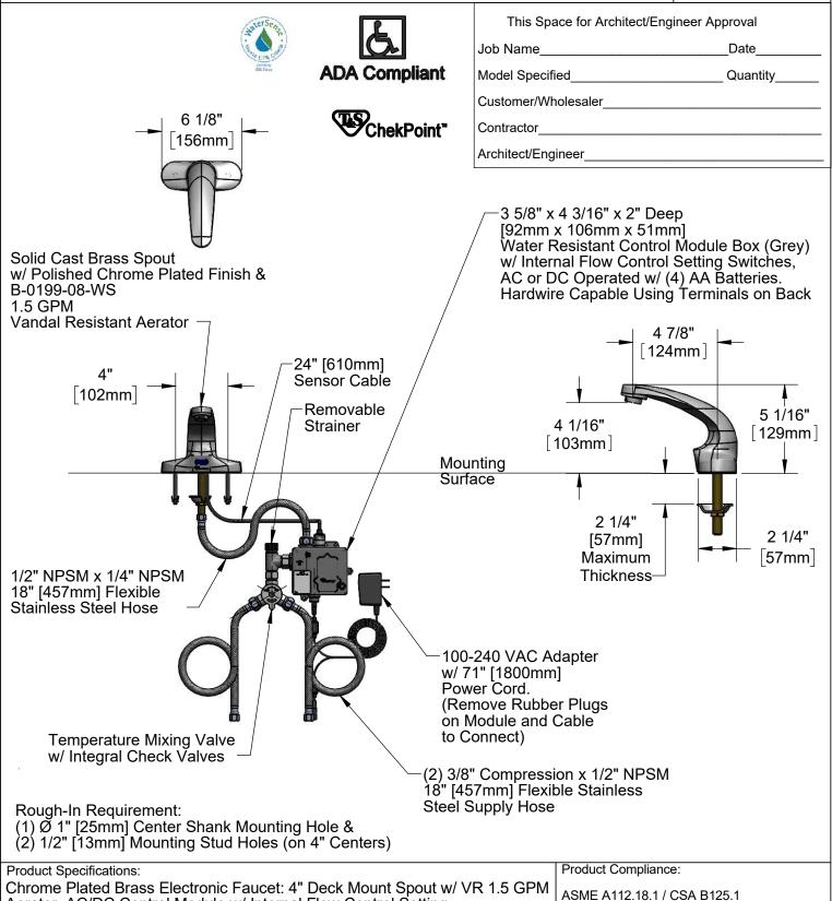
Chrome Plated Brass Electronic Faucet: 4" Deck Mount Spout w/ VR 1.5 GPM Aerator, AC/DC Control Module w/ Internal Flow Control Setting Switches, Temperature Control Mixing Valve w/ Integral Check Valves, 18" Flexible Stainless Steel Supply Hoses
