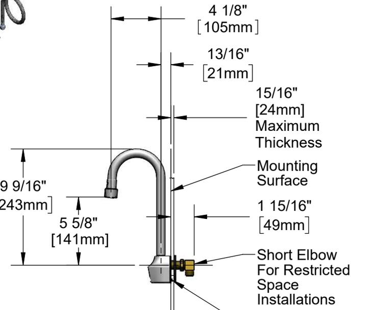
Unscrew Set Screw in Body To Desired Height for Anti-rotation Feature. (See Mounting Hole Detail)
