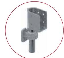
**Bottom Hinge** – For additional strength and durability the hinge is designed with pillow block constructed of zinc plated ductile iron (stainless steel is optional) with a UHMW sleeve and solid cast aluminum lower hinge adapter. Plus the lower hinge adapter has a provision for mounting an optional spring assist.
