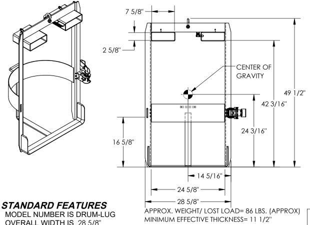
NEVER EXCEED LOAD CENTER RATING PER FORK TRUCK MANUFACTURER'S GUIDELINES. DO NOT USE THIS FORK TRUCK ATTACHMENT IF LOAD WILL EXCEED FORK TRUCK
