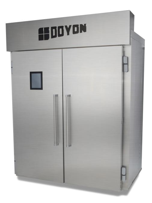
Knock Down Retarder Proofer Cabinet, Roll-In, Two-Section, Capacity (2) Double Side Load, (3) Single End Load Rack or (4) Single Side Loaf Racks, (2) Doors with Digital Touchscreen Control, Single Water Line, Auto Fill Humidity, R134A, Insulated Panels, Stainless Steel Construction, Expandable, Shipped Knocked Down, ETL, NSF
