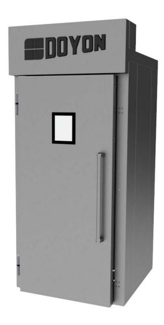
Knock Down Retarder Proofer Cabinet, Roll-In, One-Section, Capacity (1) Double Side Load/Single End Load Rack or (2) Single Side Loaf Racks, (1) Door with Digital Touchscreen Control, Single Water Line, Auto Fill Humidity, R134A, Insulated Panels, Stainless Steel Construction, Expandable, Shipped Knocked Down, ETL, NSF
