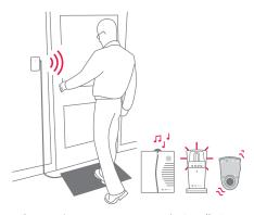
3. Step on the contact mat to test the installation. When the contact mat is pressed, it activates the transmitter that signals your Visit receiver. The receiver alerts you with sound, flashes or vibrations (depending on the receiver).
