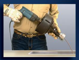
With a capacity of 50 ft. of 1/4" or 5/16", and up to 35 ft. of 3/8" Flexicore® cable, the PD-25 Auto Handy easily clears clogs in sink, shower, toilet, and laundry drain lines from 1-1/4" to 3" in diameter.
