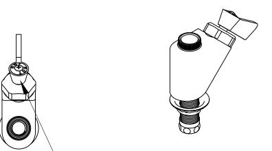
QUARTER TURN CERAMIC DISC CARTRIDGES WITH CHECK STEMS AND COLOR **CODED INDEXES**
