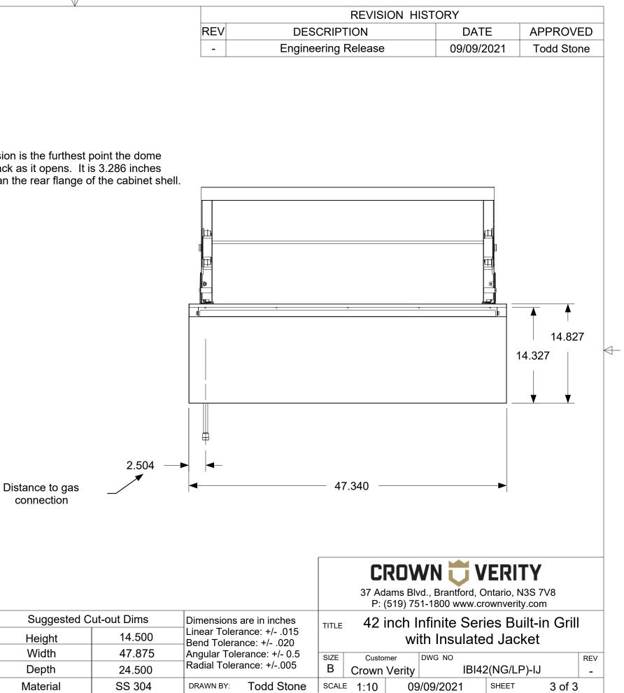
The dimensions shown are the actual physical dimensions of the grill. Additional clearances to cabinetry are dependent on the tolerances of the cut-out. The suggested cut-out dimensions are listed in the chart below but these dimensions can be reduced if the tolerances are controlled.
