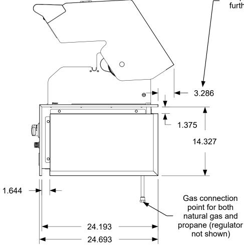
This dimension is the furthest point the dome protrudes back as it opens. It is 3.286 inches further back than the rear flange of the cabinet shell.
