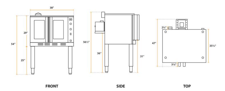
Cooking Performance Group FGC-100-DDL Deep Depth Single Deck Full Size Liquid Propane Convection Oven with Legs - 60,000 BTU
