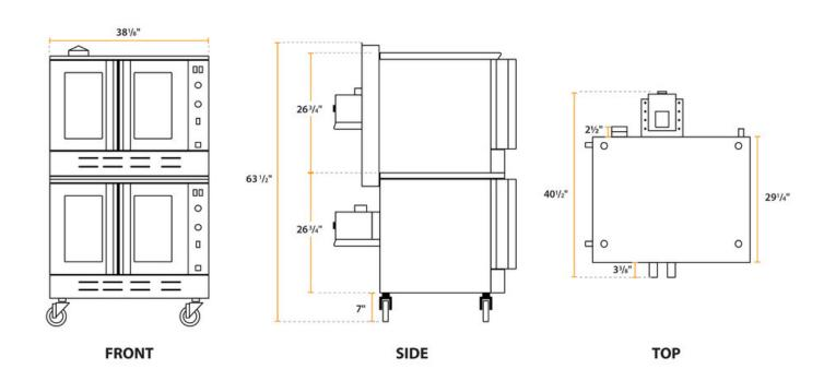
Cooking Performance Group FEC-200-DK Double Deck Standard Depth Full Size Electric Convection Oven - 240V, 1 Phase, 11.9 kW
