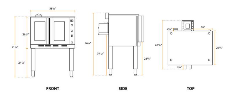
Cooking Performance Group FEC-100-C Single Deck Standard Depth Full Size Electric Convection Oven -208V, 3 Phase, 11 kW
