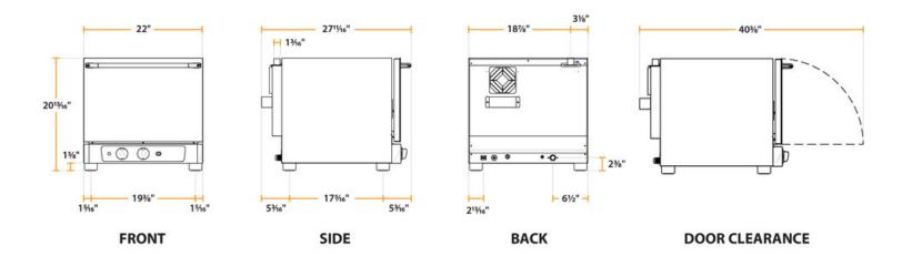
Cooking Performance Group COH-D4-M Electric Digital Countertop 4 Tray Half Size Convection Oven with Moisture Injection - 208-240V, 2700W
