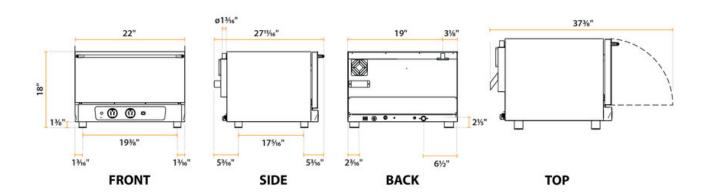
Cooking Performance Group COH-D3-A Electric Digital Countertop 3 Tray Half Size Convection Oven with Moisture Injection - 120V, 1650W
