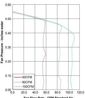
Fan Flow Rate - CFM Standard Air
