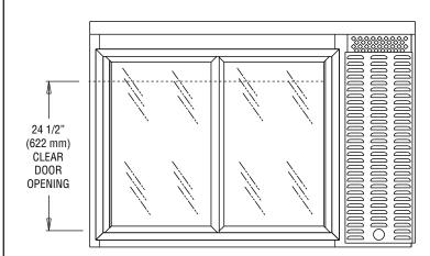
**IMPORTANT NOTE:** Models are completely front breathing and take in and exhaust air through the front grill. For proper operation, the area in front and back of the cabinet **must** not be obstructed in any way. A clearance of 3" on the sides is recommended.
