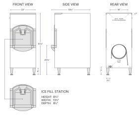
INSTALLATION NOTE: ALLOW 6" SPACE AT LEFT, BACK, AND RIGHT SIDES FOR VENTILATION AND UTILITY CONNECTION
