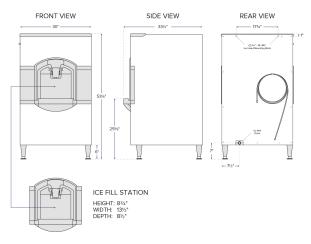
INSTALLATION NOTE: ALLOW 6" SPACE AT LEFT, BACK, AND RIGHT SIDES FOR VENTILATION AND UTILITY CONNECTIONS
