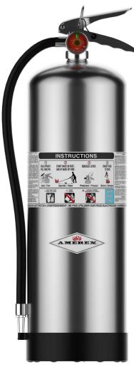
MODEL 240 utilizes the cooling, soaking, and penetrating effect of a 45- to 55-foot stream of WATER. The 55-second discharge time makes it very effective for inexperienced operators for use on Class A fires that include combustibles such as wood, cloth, paper, and many plastics. This extinguisher is constructed with a chrome-plated brass valve and polished stainless steel cylinder, which helps eliminate corrosion.
