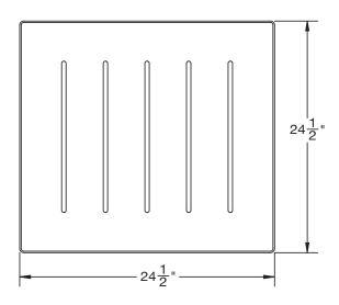
**General:** Furnish and install as shown on plans DURAPAN™ Washing Machine Pan, Model 95, as manufactured by E. L. Mustee & Sons, Inc. One-piece molded Structural Thermoplastic. Shoulder will be no less than 2 1/4" high. Shall include drain assembly for connection to 1" 90 degree PVC elbow drain fitting. Color: White.
