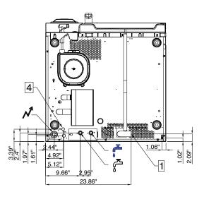
Drain Drain outlet at 2.1" from the support 29.3 - 36.3"\* from the floor
