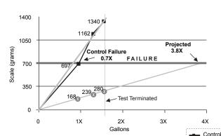
Actual field-tested from a commercial coffee brewer in 25-grain incoming hard water. The control in this side-by-side test received no treatment. CUNO SF18-S scale inhibitor was added to the feed water in the treated brewer.
