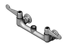
Swivel Outlet Accepts equip Swing Nozzles. Rigid Conversion Requires 014200-45 Lock Washer (Sold Separately) Ceramic Cartridges & equip 4" Wrist Action Handles w/ Color Coded Screws 2 3/8" 61mm 3" [77mm] 8" Ø 2" [51mm] [203mm] Flanges w/ Mounting Surface 1/2" NPT Adjustable From 7 3/4" to 8 1/4" Female Inlets [197mm to 210mm]
