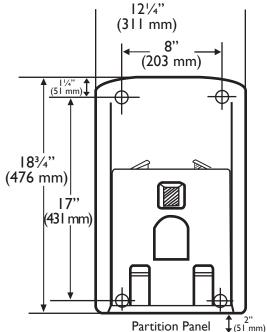
Mount 2" (51 mm) from bottom of door or 14" (356 mm) from floor
