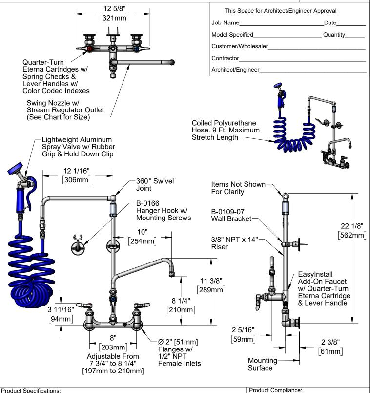
Pet Grooming Station: 8" Wall Mount Mixing Faucet, Quarter-Turn Eterna Cartridges w/ Spring Checks, Lever Handles, Add-On Faucet, 10" Swing Nozzle w/ Stream Regulator Outlet, Overhead Swivel Arm, 9' Coiled Hose w/ Angled Aluminum Spray Valve, Wall Bracket, Hanger Hook & 1/2" NPT Female Inlets
