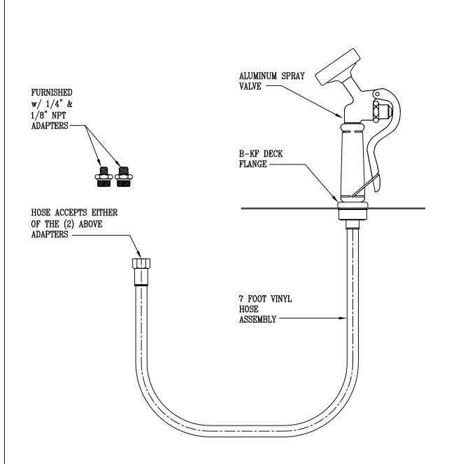
7 FOOT VINYL HOSE & ALUMINUM SPRAY VALVE WITH PROTECTIVE DECK FLANGE
