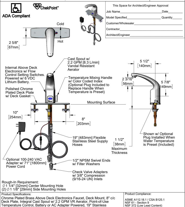
Steel Flexible Supply Lines & 3/8" Compression Inlets
