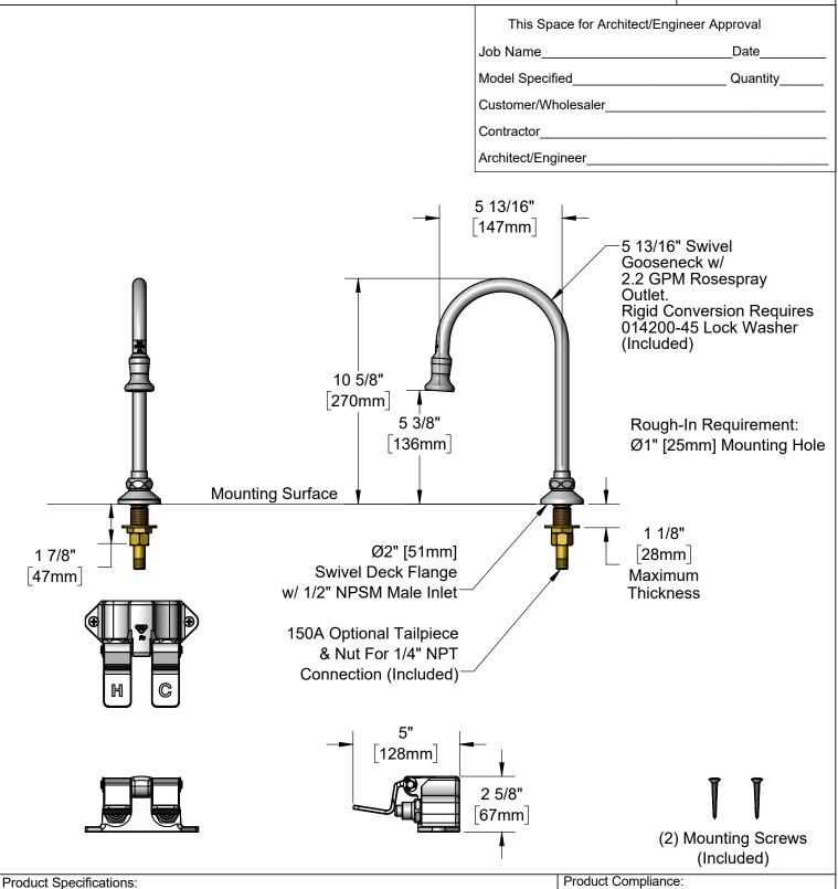
5" Dummy Gooseneck w/ Swivel Deck Mount Flange, 2.2 GPM Rosespray Outlet and Double Foot Pedal Valve w/ Fast Self-Closing Cartridge
