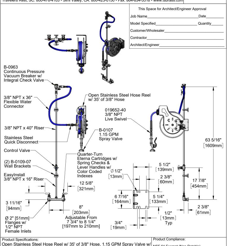
Open Stainless Steel Hose Reel w/ 35' of 3/8" Hose, 1.15 GPM Spray Valve w/ Swivel, Vacuum Breaker, 3/8" NPT Flexible Water Connector, 8" Wall Mount Mixing Faucet & Control Valve
